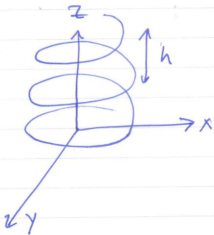
The pitch of the helix is defined as the z-distance gained through one revolution, i.e. in time
