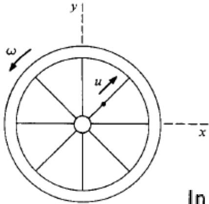
A bead moves along the spoke of a wheel at constant speed  $u$  meters per second. The wheel rotates with uniform angular velocity  $\dot{\theta} = \omega$  radians per second about an axis fixed in space. At  $t = 0$  the spoke is along the  $x$  axis, and the bead is at the origin. Find the velocity at time  $t$
