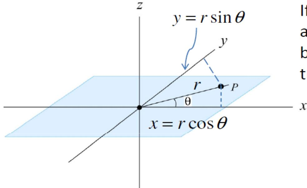
If polar coordinates  $(r, \theta)$  of a point in the plane are given, the Cartesian coordinates  $(x, y)$  can be determined from the coordinate transformations
