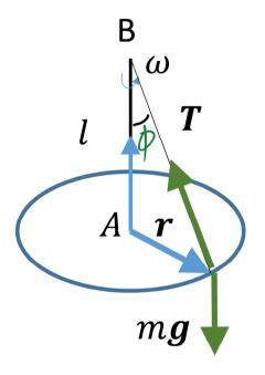
The pendulum is in steady circular motion with constant angular velocity  $\omega \hat{k}$ .
