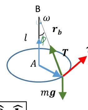
The pendulum is in steady circular motion with constant angular velocity  $\omega \hat{k}$ .
