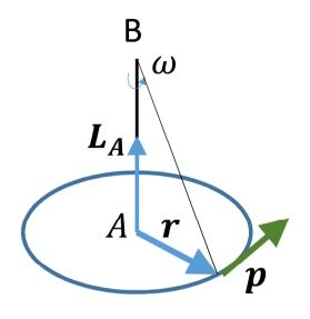
The pendulum is in steady circular motion with constant angular velocity  $\omega \hat{k}$ .
