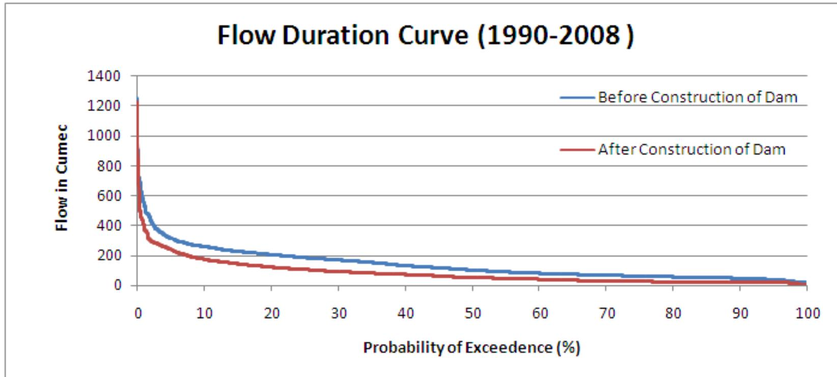
Flow duration curve before and after construction at Dam site
