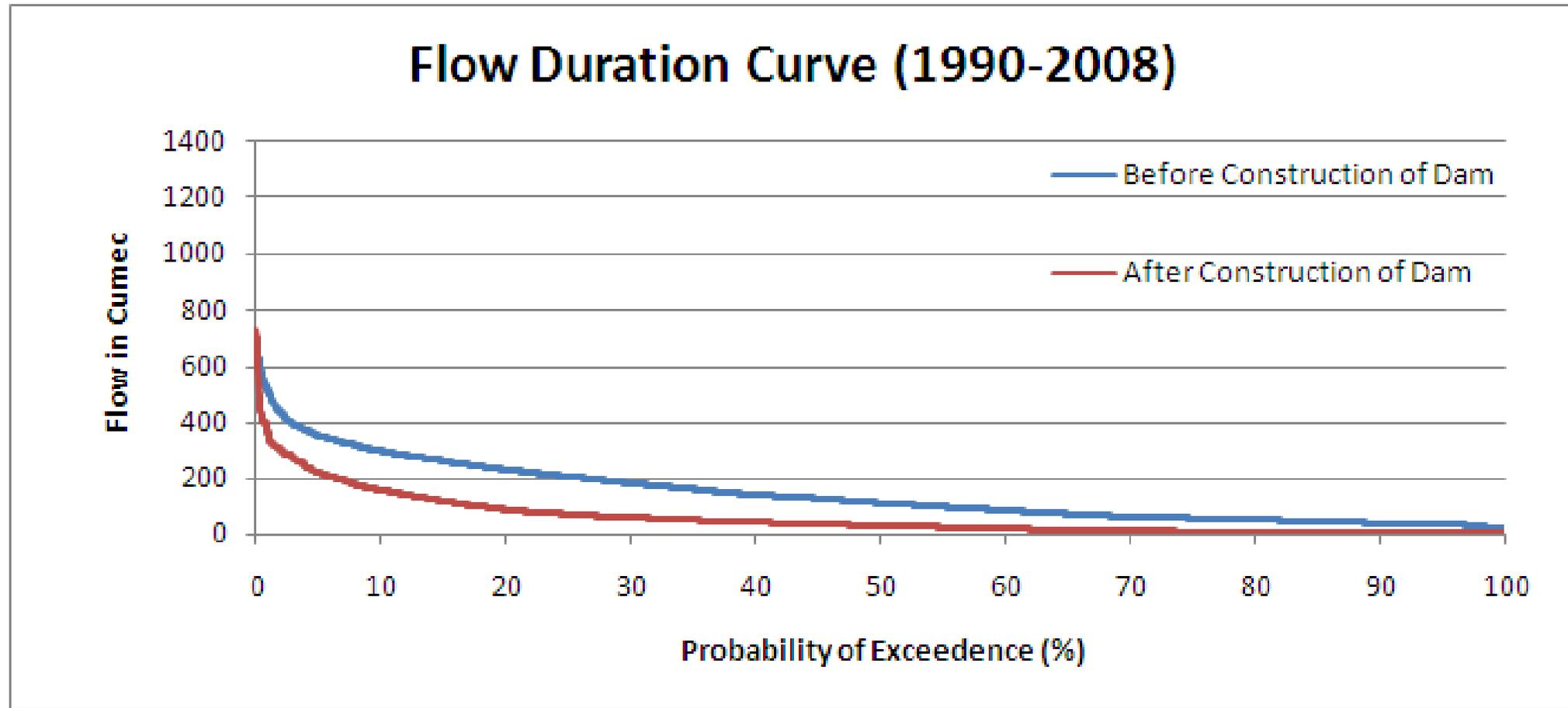
Flow duration curve before and after construction at NH crossing
