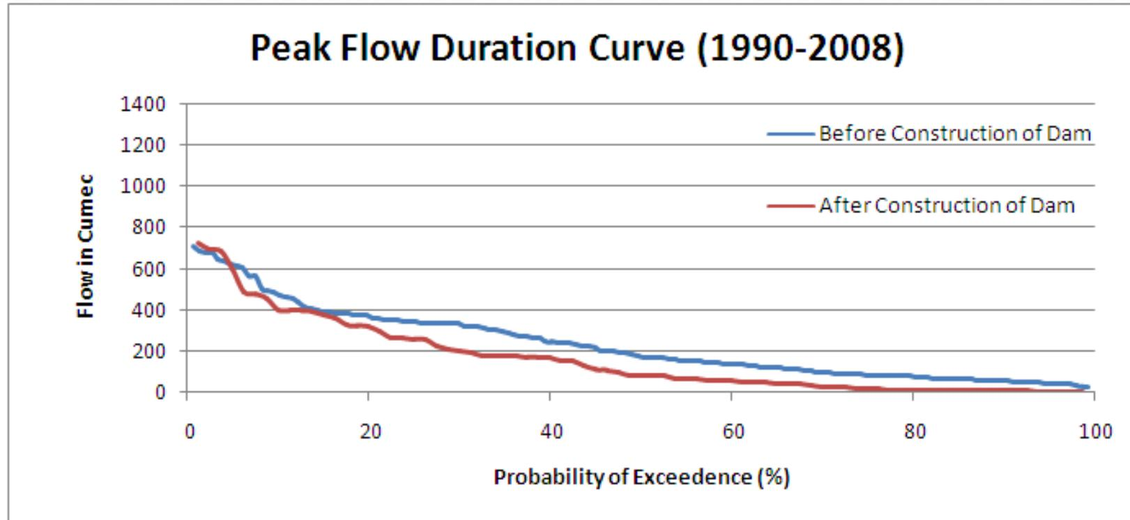
Monthly peak flow duration curve before and after construction at NH crossing
