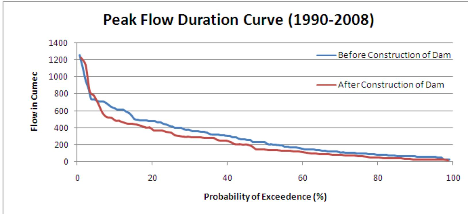
Monthly peak flow duration curve before and after construction at Dam site
