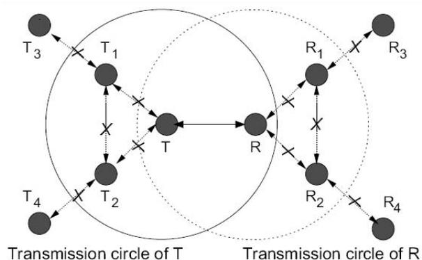
Fig. 1. Interference model for a bi-directional transmission ( $T \rightarrow R$ )
