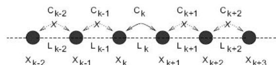
Fig. 2. Constraints representing the simultaneous service of calls in a WLN-1 network.
