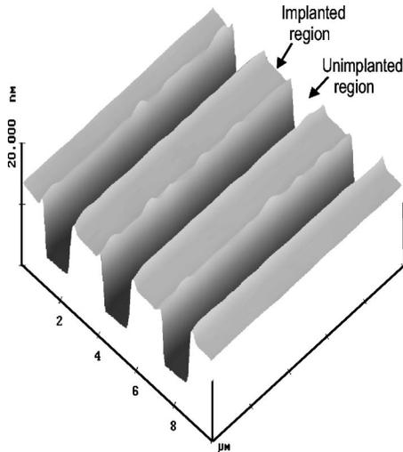
FIG. 1. An AFM image of the swelling observed in 80 keV  $\text{Si}^+$  implanted Si at room temperature, with fluence  $6 \times 10^{15}$  ions/cm<sup>2</sup>. Unimplanted region corresponds to masked region during implantation.
