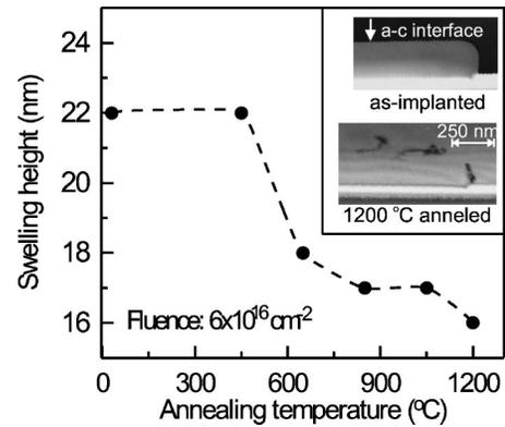
FIG. 2. The saturated step height as a function of post-implantation isochronal annealing at various temperatures, shown for  $6 \times 10^{16}$  ions/cm<sup>2</sup> implanted sample. Inset shows the XTEM images of the as-implanted and 1200 °C annealed samples, respectively.
