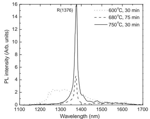
Fig. 4. PL spectra of p-type CZ Si implanted with  $1.2\text{ MeV Si}^+$  ions to a fluence  $2 \times 10^{13}\text{ cm}^{-2}$  and annealed at various temperatures.
