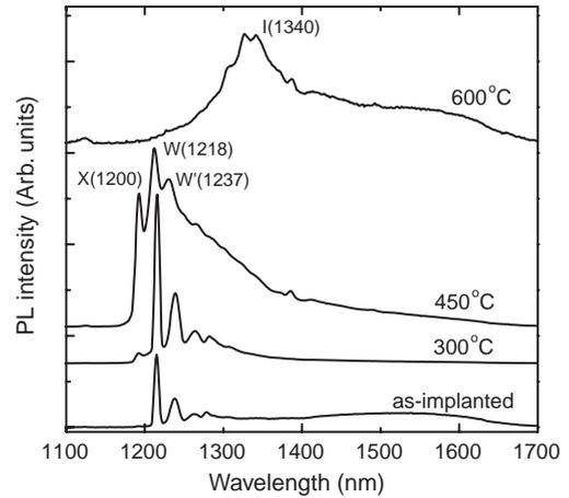
Fig. 1. PL spectra of n-type epitaxial Si implanted with 80 keV  $1 \times 10^{14} \text{ cm}^{-2}$  Al<sup>+</sup> ions followed by post-implantation annealing for 1 h at various temperatures. The spectra are scaled appropriately and shifted upward vertically for clarity.
