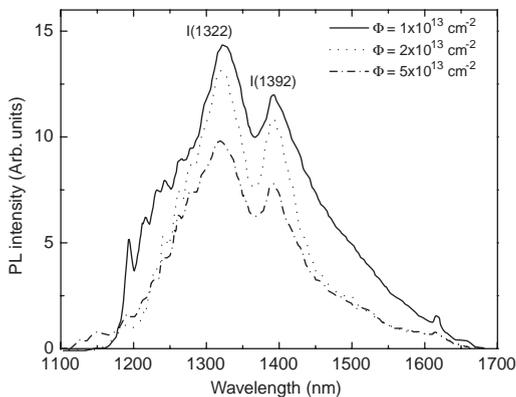
Fig. 2. PL spectra of n-type CZ Si implanted with  $1.2\text{ MeV Si}^+$  ions to various fluences ( $\Phi = 1 \times 10^{13}$ – $5 \times 10^{13}\text{ cm}^{-2}$ ) and annealed at  $600^\circ\text{C}$  for 4 h in nitrogen ambient.
