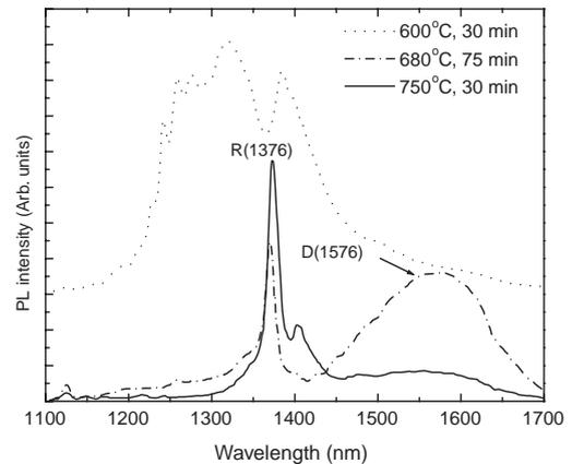
Fig. 3. PL spectra of n-type CZ Si implanted with  $1.2\text{ MeV Si}^+$  ions to a fluence  $2 \times 10^{13}\text{ cm}^{-2}$  and annealed at various temperatures.
