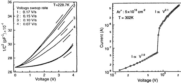
**Fig.2. (a)** C-V characteristics with decreasing and increasing bias showing hysteresis effect in Au<sup>+</sup> implanted n-Si. Arrows indicate the direction of voltage sweep and different set of curves were obtained for different degrees of bias injection. **(b)** Forward I-V characteristics of irradiated sample showing ohmic and space charge limited current regions.
