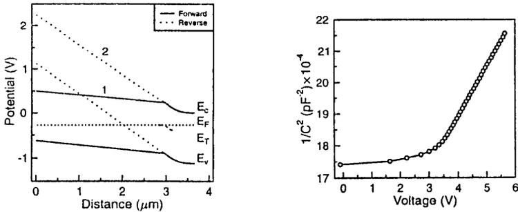
**Fig.4.** Typical calculated (a) energy band diagram and (b) corresponding simulated C-V characteristics for a Schottky diode with one midgap acceptor trap level at energy  $E_T$ .
