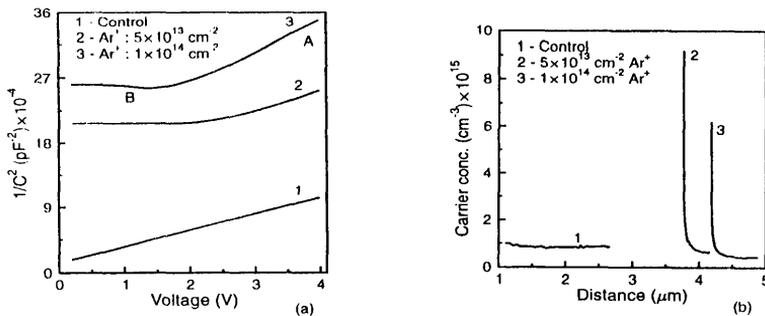
Fig.1(a) Typical C-V characteristics at 300K for n-Si Schottky diode before and after irradiation with various doses of Ar<sup>+</sup> ions.(b)Apparent carrier concentration profile obtained of curves of (a)
