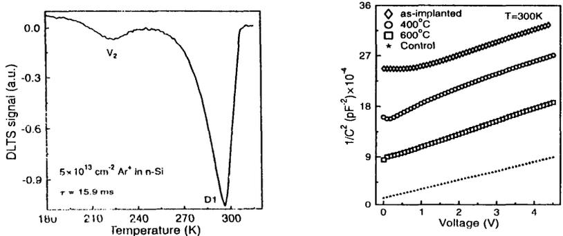
**Fig.3. (a)** A typical DLTS plot of Ar<sup>+</sup> irradiated sample showing divacancy V<sub>2</sub> and midgap acceptor D1. **(b)** Comparison of C-V characteristics at 300K of unimplanted, as-implanted and n-Si. The implantation dose was 5x10<sup>13</sup> ions /cm<sup>2</sup>.
