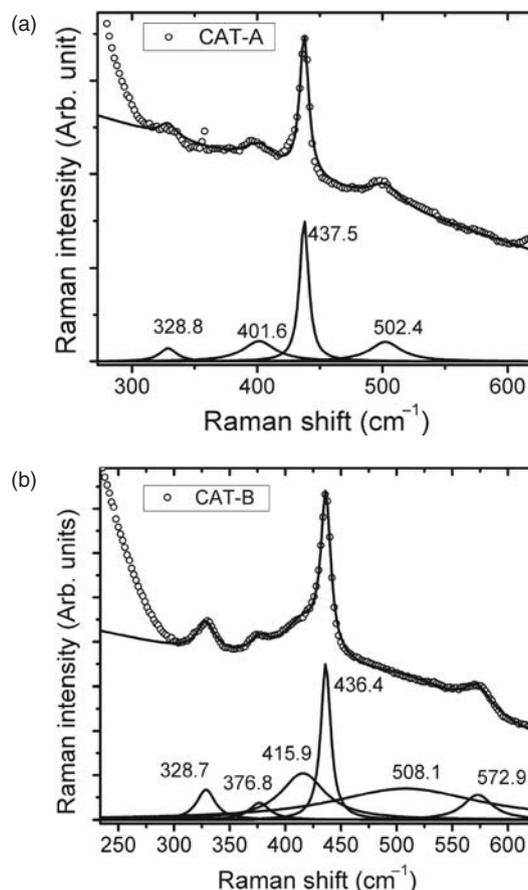
**Fig. 6.** Raman spectra of (a) CAT-A and (b) CAT-B samples. Constituent peaks are fitted with Lorentzian line shape after background subtraction.
