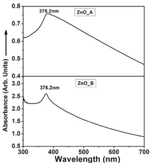
**Fig. 4.** UV-vis absorption spectra of CAT-A and CAT-B.
