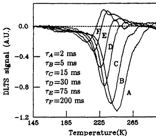
Figure 1. DLTS spectra of Si irradiated with  $\text{Ar}^+$  at dose  $1 \times 10^{14}$  cm<sup>-2</sup> showing negative peak for slower rate windows.
