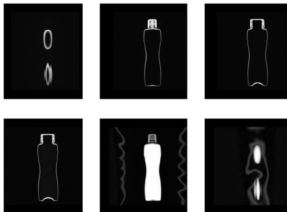
Fig. 2. Six slices of the “Blue small” container in the coronal plane
