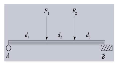
$$R_A = \frac{(F_1 + F_2)d_3 + F_1d_2}{L} = \frac{F_1(d_3 + d_2) + F_2d_3}{L}$$
