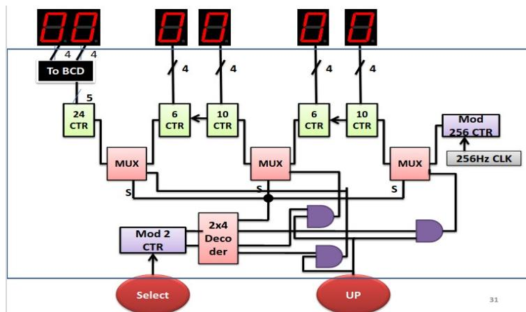
Implement any behavioral model (using +, mod operations) **and/or** structural model (using FFs, Gates and interconnection) **and/or** data flow model for your counters/mux/bcd unit/. Also try to use automatic (utomatic clock available in the FPGA board (you may need to scale down to 1Hz) or manual clock (using switches). Automatic clock have higher weight-age.
