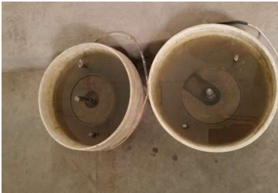
Fig.4 CBR sample in soaked condition under thawing process
