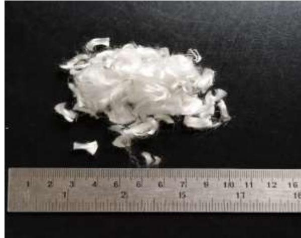
Fig.2 Discrete PP fibers used for soil reinforcement
