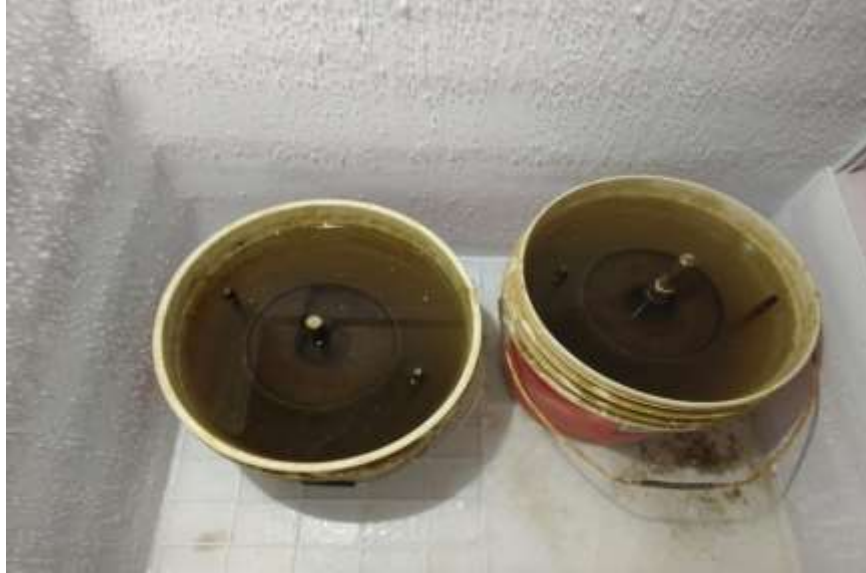
Fig.3 CBR sample in soaked condition under freezing process
